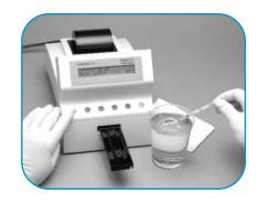
**3 Blot** the strip to remove excess urine by *touching the edge* to a paper towel. Do not drag the strip across the towel; touch the edge only.
