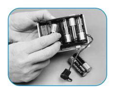
Turn the instrument over and snap the battery pack into the opening.
