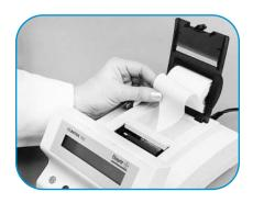
3 Pulling toward the back, gently pull the end of the paper until the full width of the paper is completely exposed.
