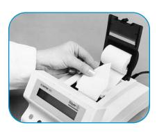
Feed the paper through the printer cover opening and snap the cover into position.
