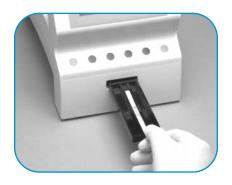
5 The table is automatically pulled into the instrument for reading. Results are available in one minute. Be sure not to move or bump the table.
